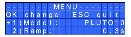
1) **Model**: you can select the screwdriver to be used. Your choice will automatically change the default settings. It's important to select the correct model you're going to use since many parameters regarding the motor software are specific for every single model.
