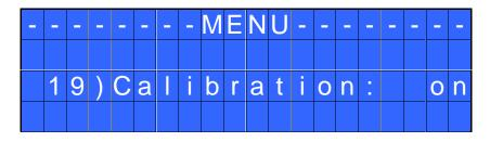
3. Press OK to confirm. If you choose OFF, calibration will be interrupted and no torque value will be displayed. You choose ON, calibration will continue and the following screen will be displayed:
