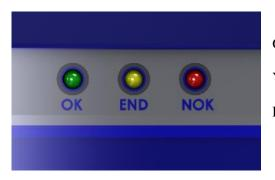
GREE LED: *Screw OK*. YELLOW LED: *Program End* (only on *EDU 2AE/HPro*). RED LED: error.
