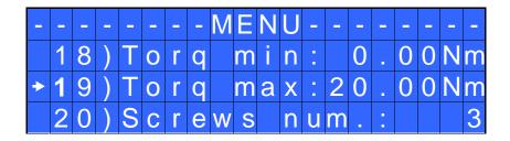
**18)** Torq min – Minimum torque: The minimum torque and maximum torque options allow the user to set the acceptable torque range for each single application. When the reached torque is inside this range, "tightening OK" will be displayed on the status bar and the green led will light up. If the reached torque is outside this range the messages "error minimum torque" or "error maximum torque" will be displayed. You can set the torque range from 0 to 40 Nm at intervals of 0.01 Nm.
