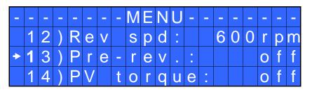
**12) Rev speed – Reverse speed:** You can select any reverse speed value of the screwdriver between the maximum and the minimum specific speed of every single screwdriver (see table with technical data).
