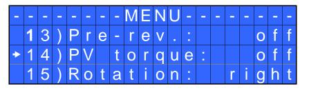
14) PV torque: Period of time in which the screwdriver works at maximum torque before switching to the torque that has been set by the user. You can set time from 0.1 to 10.0 sec. To disable the function select OFF by pressing  $\mathcal{D}$  as many times as needed.
