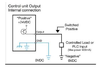
These pins can be used directly connected to PNP inputs (PLC) or used to turn on LEDs, buzzers or other devices with 24V power supply. The maximum total power of the outputs is about 400mA. Using inductive loads such as relays or other loads with an initial consumption peak greater than 400mA will send all outputs to protection, displaying the message "output disable". To restore the outputs after a protection, turn off and turn on the unit again.
