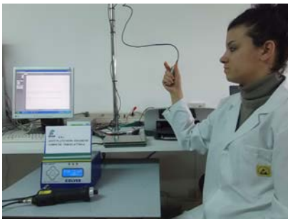
HBM Triboelectric compatibility – Operator holding probe only
