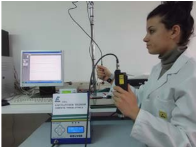
HBM Triboelectric compatibility – Operator holding screwdriver and probe
