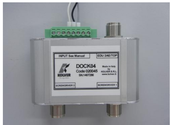
Wired DOCK04 double output connector
